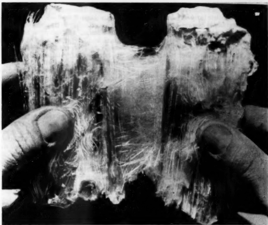
Nature's most remarkable inorganic creation — asbestos. As found in the natural rock, asbestos is dense and heavy and usually has the aspect of stone. When the silky fibers are opened up, the best grades break down into a mass of delicate, interlacing, light-colored threads which — because of their remarkable chemical and physical properties — have become indispensable to civilization. [Courtesy Johns-Manville].
